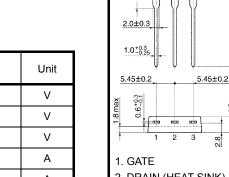
1. GATE 2. DRAIN (HEAT SINK) 3. SOURCE JEDEC — JEITA — TOSHIBA 2-16C1B
